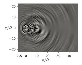
Predicted acoustic pressure field in the x-y-plane for a jet emanating from a chevron nozzle.
