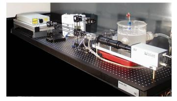
Optical set-up to apply for DPIV measurements in a
